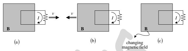
**Experiment 1:** He pulled a loop of wire to the right through a magnetic field. A current flowed in the loop (Figure a).
